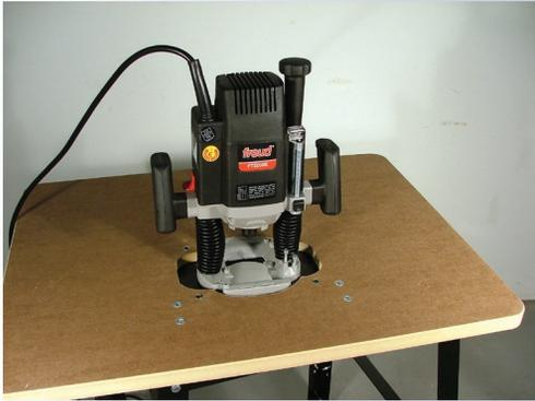
**above** It is easier to flip the top to attach the router
