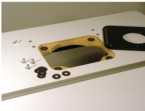
**left** Place shims in the recess to set the insert plate level with the top
