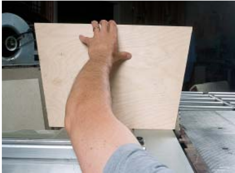
PHOTO C: The seat can be used to set the angle of the table saw blade for all of the bevel cuts on the rocker.
