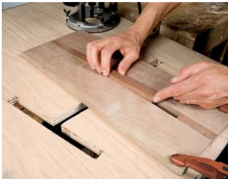
PHOTO A: A filler strip can be inserted in the interim dado jig to rout the short slot for the strut.
