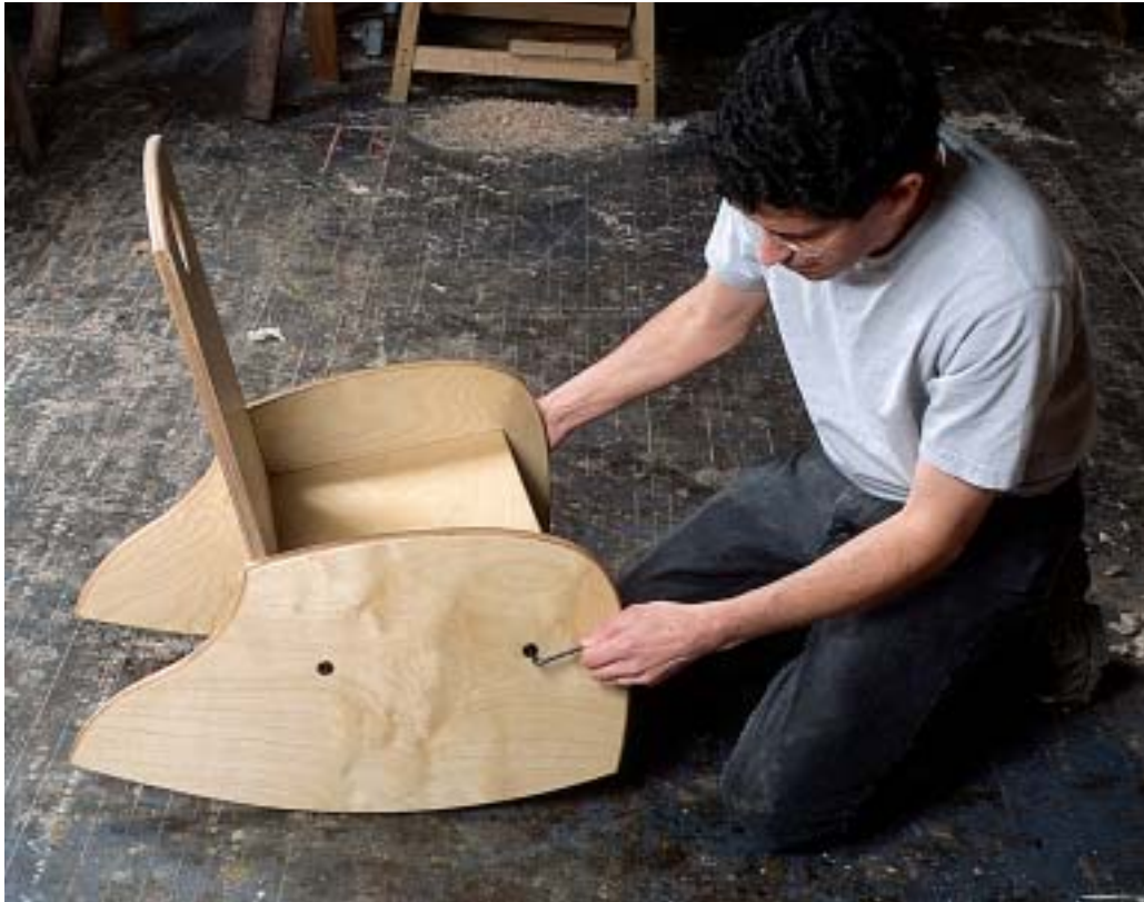
PHOTO J: Tighten up the cap nuts with a pair of Allen wrenches.
