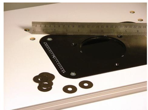
**right** When tightened down, check the insert plate is flush
