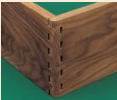
Wooden hinges (knuckle joints) are an easy variation on standard finger joints.
