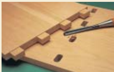
A sharp corner chisel makes short work of squaring mortises.
