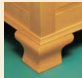
Above: Doweled bracket feet and base frame for corner of blanket chest, right.
