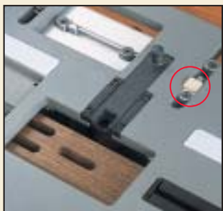
4 Move table to the left; rout front left tenon.
